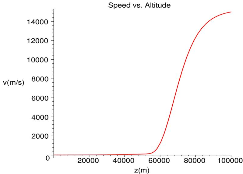
Note that, when atmospheric density is constant, the projectile slows down at a much greater altitude than for the variable density case. Naturally we would expect the greatest negative acceleration force to occur where the atmosphere is densest.
